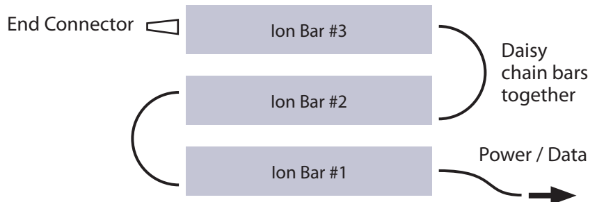
End Connector - must be plugged into the end of the last Bar
